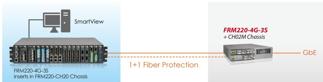
Protocols: Fast Ethernet, Gigabit Ethernet, OC-3, OC-6, OC-12, STM-1, STM-4, STM-16, FC-1, FC-2
