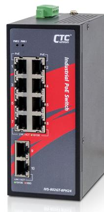
Industrial grade E-Mark certified PoE switch IVS-802GT-8PH24, with 2 Gigabit UTP ports and 8 10/100 PoE ports, input power range 24/48VDC, suitable for vehicle battery power supply. E-Mark is a European conformity mark that certifies that a vehicle or vehicle part complies with EU regulations. Laws and directives to ensure adequate safety and meet all environmental requirements for vehicle installation.
